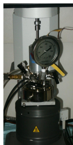
300 ml Parr reactor used in lab to produce polyolefins.
